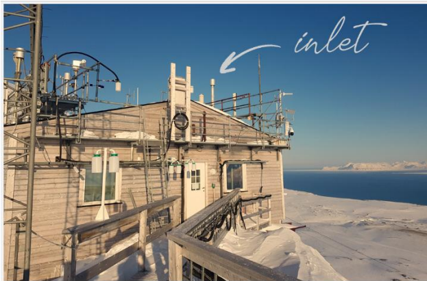
Fig 6: Zeppelin Observatory on a clear sunny day on 6 April 2022. The observatory is situated 474 metres above sea level, not quite reaching the summit of the mountain. The whole-air inlet is labelled, through this is how we sample the air.
