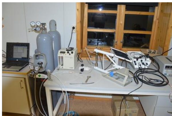
Calibration of EC150 gas analyser in the Vaskeri Lab
