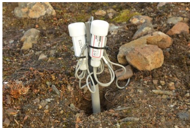
On field set up of the soli temperature datalogger in the CALM GRID area close to CCT. Photo: Angelo Viola, CNR.
