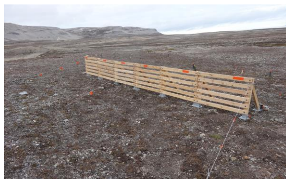
The snow fence at the dry tundra site in Knudsenheia. Turbulence will cause snow to accumulate down-wind of the fence and will enable us to study the effect of increased snow cover on the microbial communities and their ecosystem functions. Photo: Bjorn Tytgat, UGhent.
